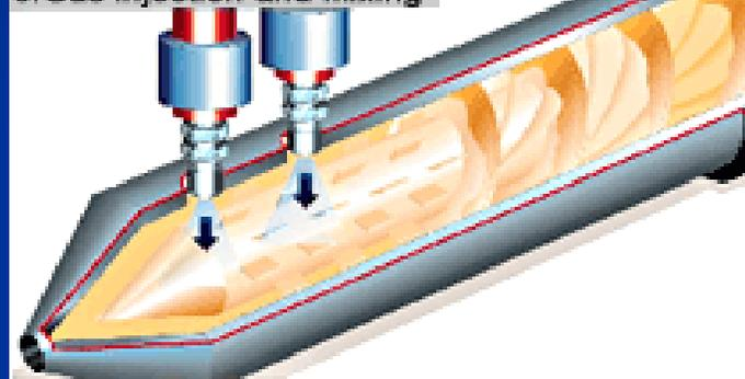
The gas is injected into the polymer melt and mixed.
