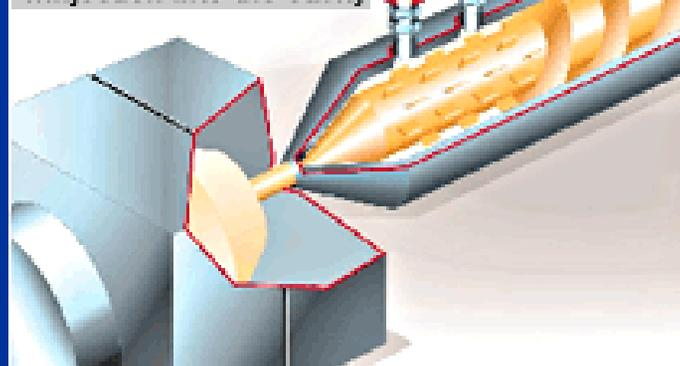
The plastics-gas mixture is under pressure and is injected into the injection moulding tool, where it forms small, finely distributed gas bubbles.
