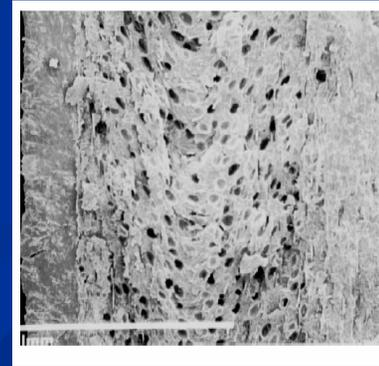
Micrograph showing average cell size of 10 microns (.0004 Inches)
