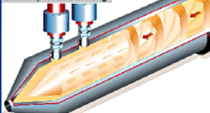
The plastic is plastified and homogenized by heating while being transported.
